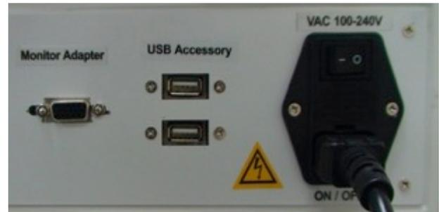
C. AC 110V/220V and ON/OFF are the main power switch and the power cord socket. The fuse chamber is in between the main power switch and the power cord socket.
