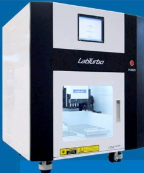
Automation for 384-well plate PCR setup
