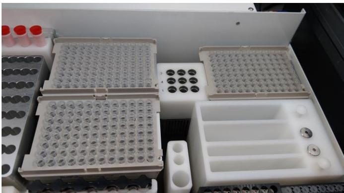
5. Carefully place 6-strip 2.0 mL sample tubes (**with samples**) on the **Sample lysis thermoblock** one by one.
