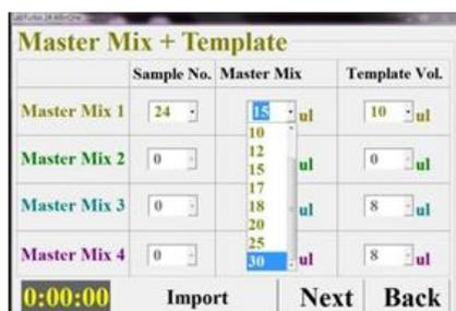
6. Select template volume. Maximal template volume is 30 uL. Minimal template volume is 2 uL.
