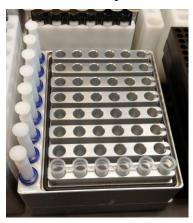
9. Place the PCR Tubes and the caps sequentially. Then put the cover of PCR tubes on the rack.
