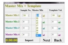
6. Select template volume. Maximal template volume is 30 uL. Minimal template
