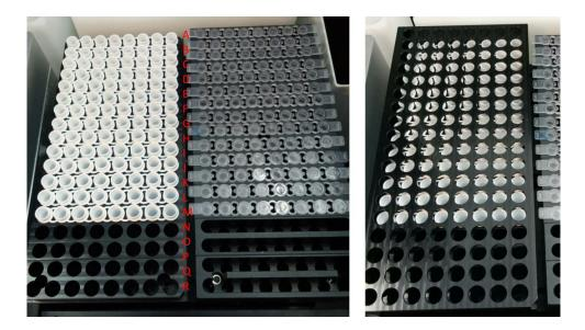
Place the qPCR reagents into the designated position of the rack.
