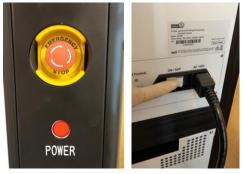
"XY/ZW/T/Heater1/Heater2 connect error, checking the RS232USB connection" This message indicates that the controller does not connect to computer. Please turn off the LabTurbo AIO 48 SP-qPCR Automation System. After all are turned off, switch the main power off and on once, and then turn on the machine again. If this message remains, please contact our customer service.
