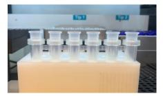
8. Insert the sample tube into the rack of **Elution vacuum manifold**.
