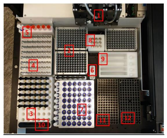
(1)Robotic arm (2)96-well Tip rack (3)Binding-washing vacuum manifold (4) Sample lysis thermoblock (5)Plug tube rack (6)Proteinase K tube rack (7)Elution vacuum manifold (8)PCR component rack (9)Buffer tank (10)Tip disposal vent (11)8-strip PCR tube rack (12)8-strip PCR tube cover rack
