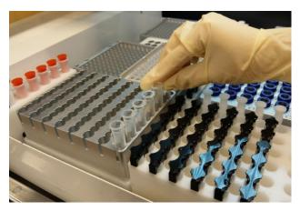
6. Remove the cap of the proteinase K vial and put it in the **Proteinase K rack**.
